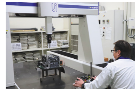
部品検査(3次元測定) Parts Inspection (3D measurement)
