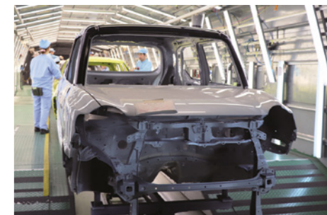
塗装(塗装検査) Painting (Painting Inspection)
